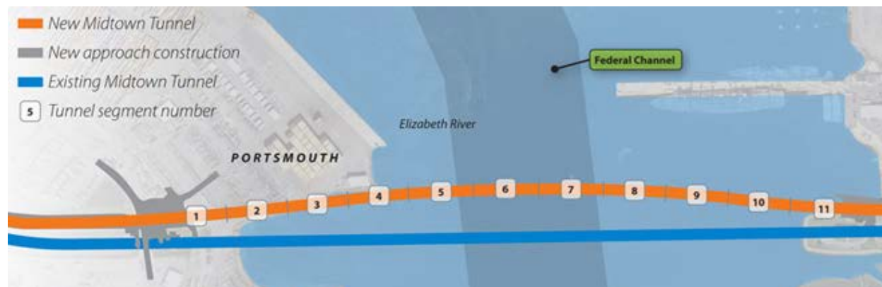
Figure II Example curvilinear ITT horizontal layout to minimize upland land impacts at the Elizabeth River Tunnels – Second Midtown Tunnel Project 65 .
