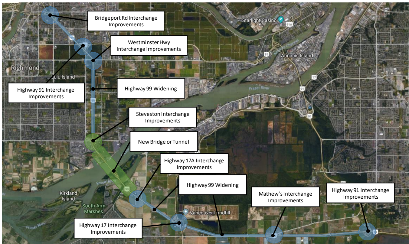
Figure 23: Extent of Do Minimum (Green) and Reference Concept (Blue) Improvements along Highway 99
