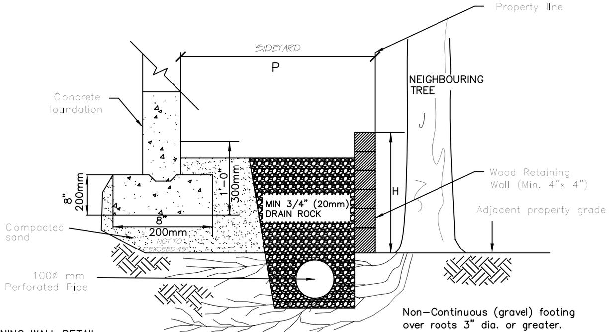
FOR WOOD RETAINING WALL DETAIL REFER TO BULLETIN BUILDING – 07.
