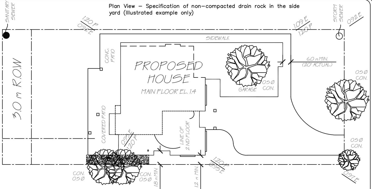
Non-compacted drain rock (min. 20mm (3/4" aggregate crushed drain rock) in the side yard (see section detail).
