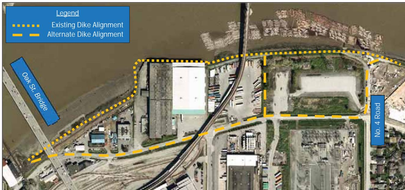
For the long term flood protection strategy, preferred adaptation is to maintain the dike alignment on the waterfront to protect all infrastructure. The Fraser River Terminal will require a site-specific adaptation at a time when the site is redeveloped, which is not anticipated in the imminent future. In the interim, the Fraser River Terminal site is considered a generally constrained area, discussed further in **Section 4.3.1**.
