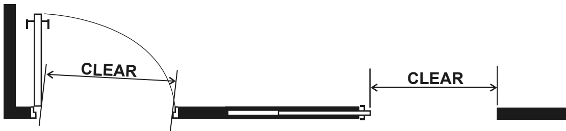
Figure 1. Clear Opening Measurement For Doors
