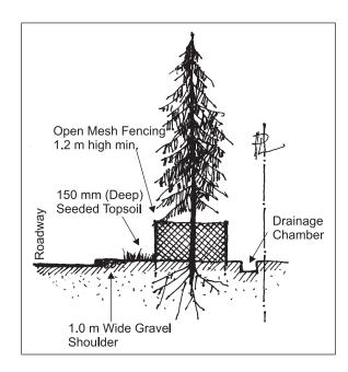
Above diagram reflects how tree fencing and gravel shoulders are to be installed.
