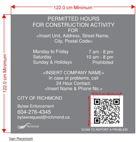
Height From Ground - maximum 3.65 m Height From Ground - minimum 1.52 m
