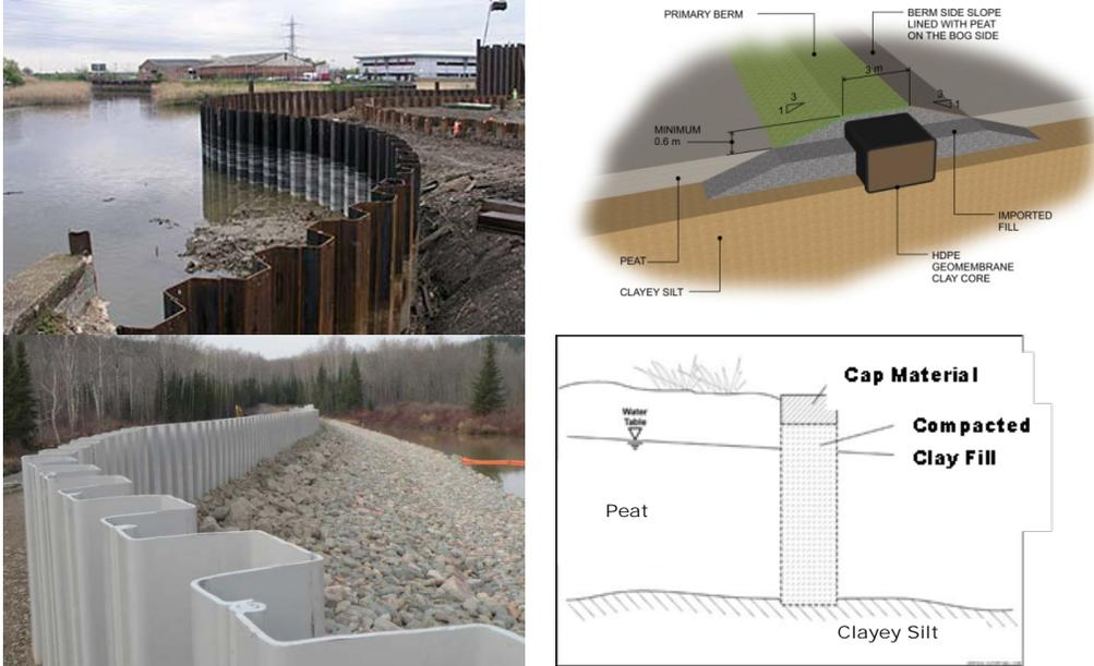
Figure 10-3: Subsurface Barrier Construction Options
