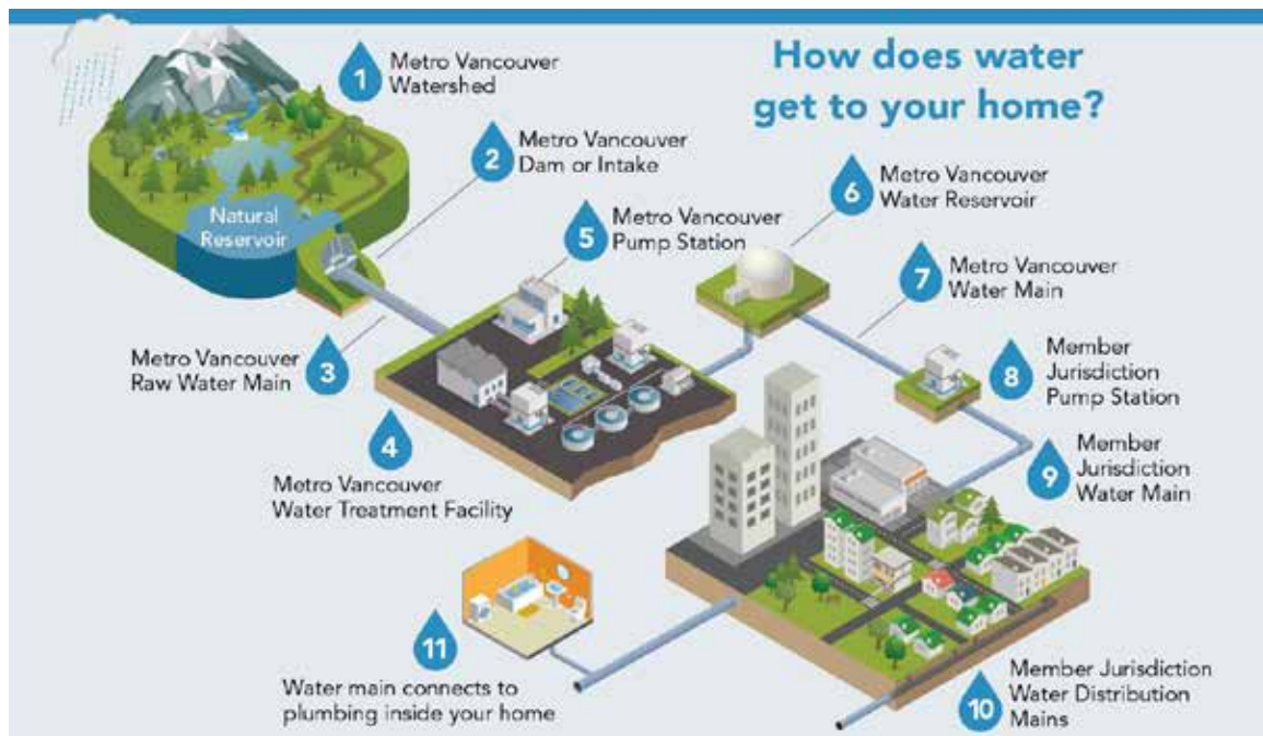
Metro Vancouver Watershed and Water Transmission Map
