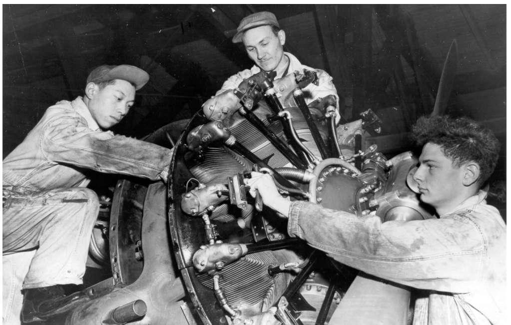
Ernie Chan, Gord Felski and Irving Beck overhaul a Harvard motor during weekend training.
